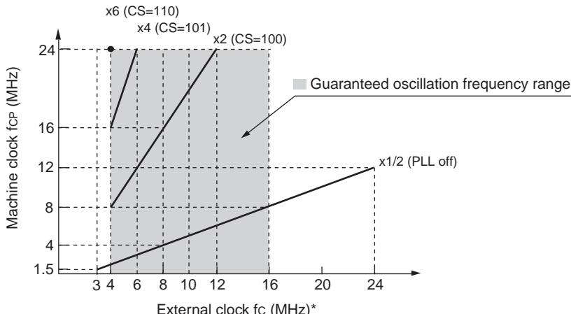
\* : When using a crystal oscillator or a ceramic oscillator, the maximum oscillation clock frequency is 16 MHz.
