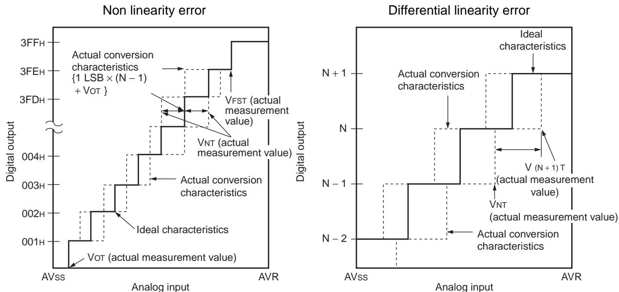
$$\text{Non linearity error of digital output } N = \frac{V_{NT} - \{1 \text{ LSB} \times (N - 1) + V_{OT}\}}{1 \text{ LSB}} \text{ [LSB]}$$
