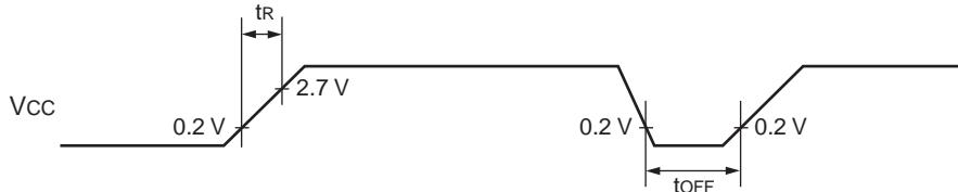
Note : If you change the power supply voltage too rapidly, a power-on reset may occur. We recommend that you start up smoothly by restraining voltages when changing the power supply voltage during operation, as shown in the figure below. Perform while not using the PLL clock. However, if voltage drops are within 1 V/s, you can operate while using the PLL clock.
